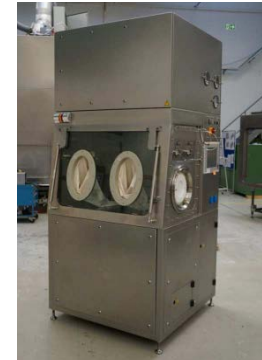
Connecting Isolator Mobile unit from process to process
