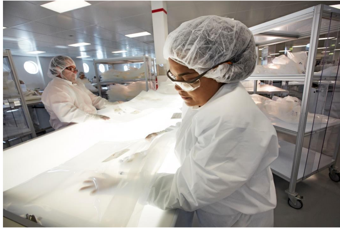
Light table (transmission) at 1900 lux, 35 second inspection time See Wormuth et al, PDA Journal 2021 Vol 75 page 332 ASTM Standard under development: E55 WK87243
