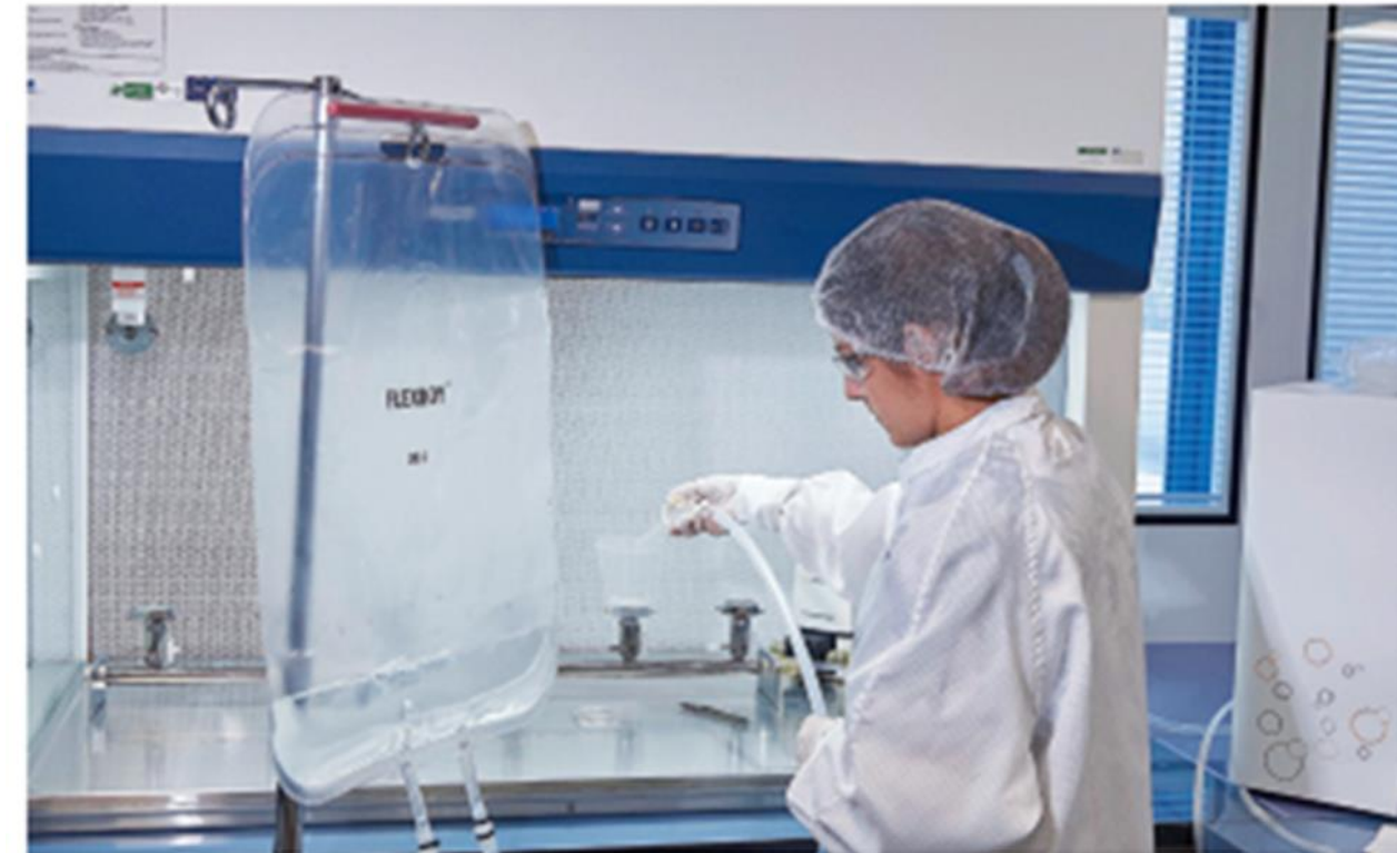
Extraction with water and measurement via automated membrane microscopy See Wormuth et al, PDA Journal 2024 Vol 78 page 90 Relevant ASTM Standards E3230, E3411, E3425, E3466, E3468
