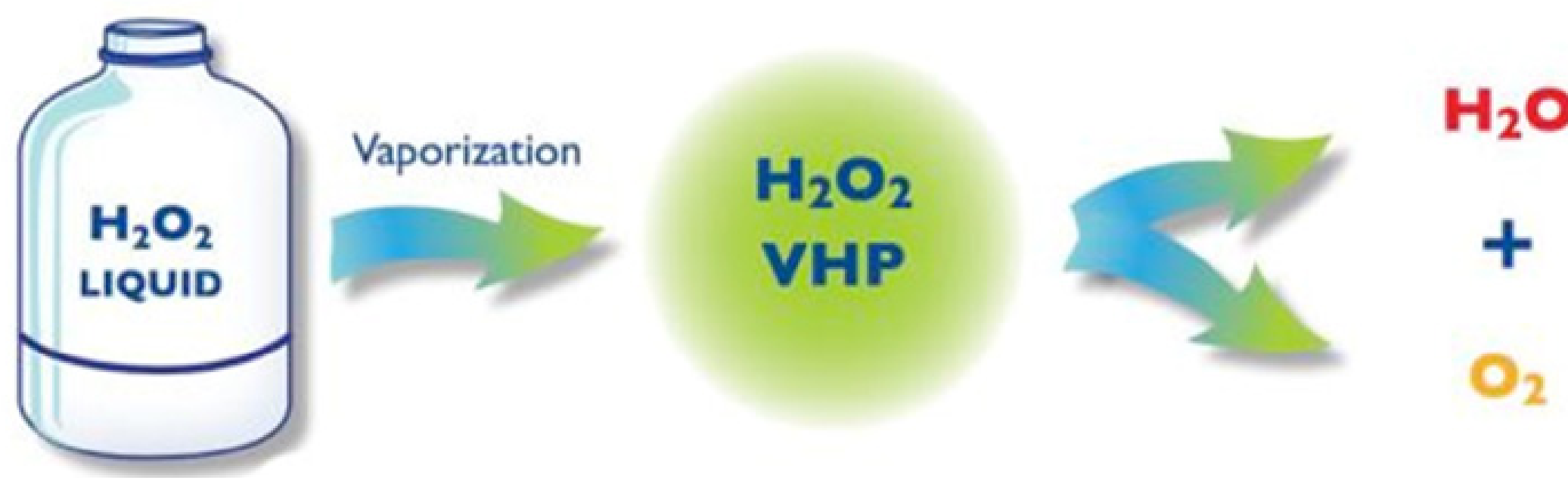
Figure 4: Depiction of Liquid H2O2 Vaporizing and Post Application VHP Breakdown into Water Vapor and Oxygen
