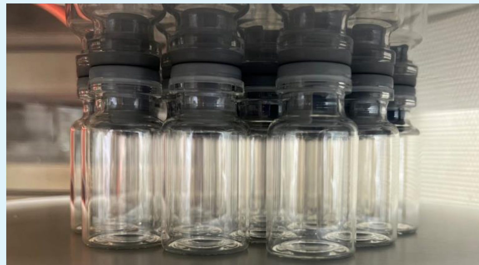
Stoppers Compressed into Glass Vials by Chamber Plates
