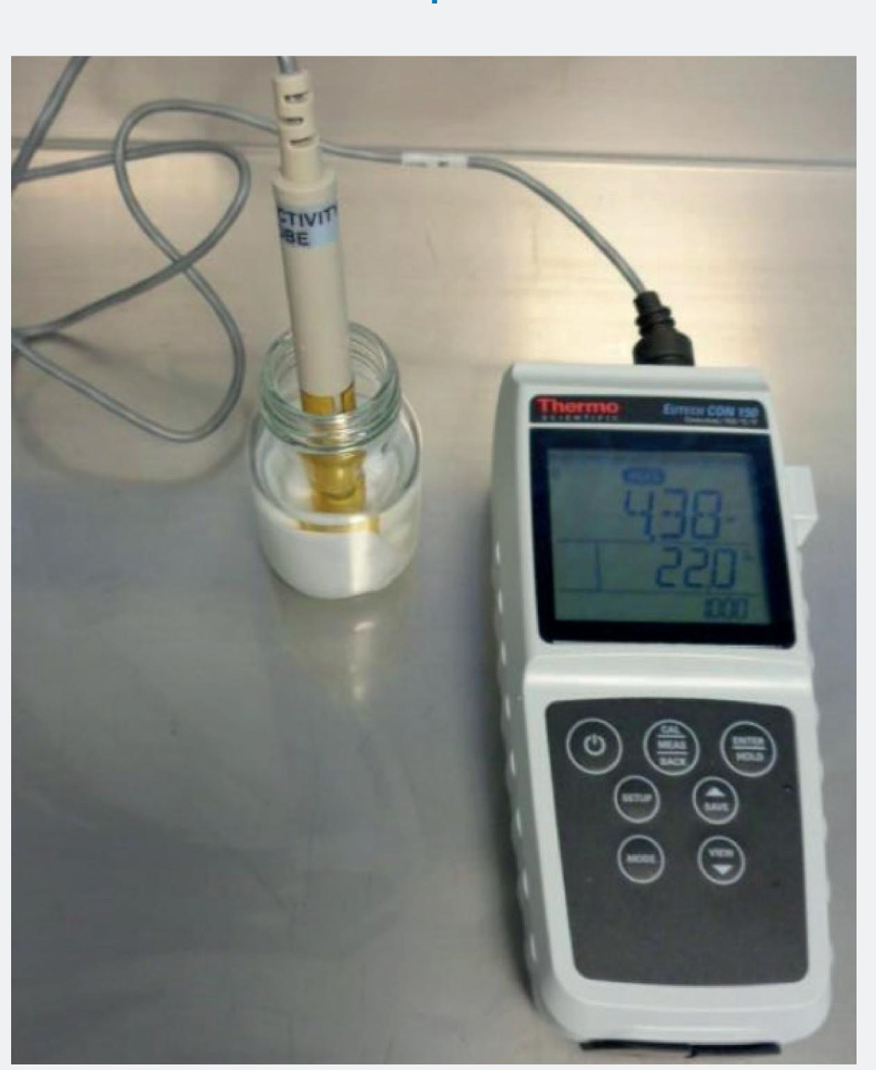
Figure 1 - Conductivity of a 300 x 300 mm 45% polyester and 55% cellulose wipe in KWI. Typical values should be ideally below  $< 10 \pm 2 \mu \text{S/cm}$ . The example shows 4.38 µS/cm for the chosen wipe and water quality selected.
