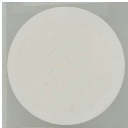
Figure 1 Filter Showing a Low Level of Metformin Contamination (Manufacturer A)
