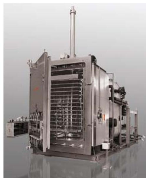
**Figure 1** A Typical Industrial-scale Pharmaceutical Batch Freeze-dryer
