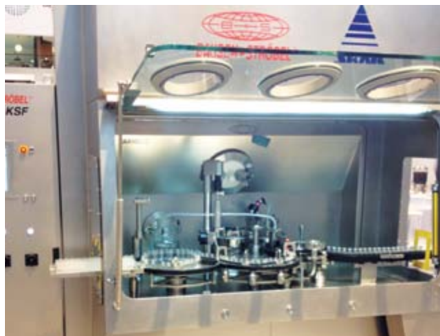
Pictured above is SKAN’s modular single chamber isolator PSI-L with a Bausch+Stroebel Variosys vial filler. Photo courtesy of SKAN
