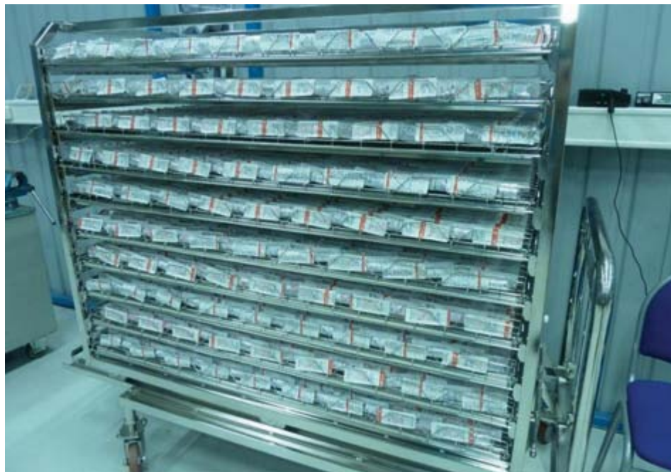
This is a typical loading cart configuration with an array of specified products for sterilization
