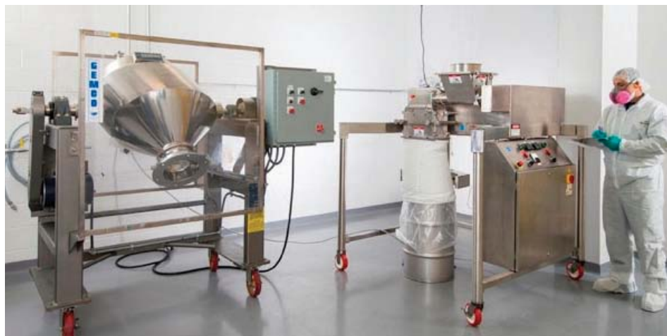
Photo courtesy of by Jim Greipp of Pau Hana Productions for Custom Processing Services. This photo depicts a cleanroom/ flexible processing station showing a slant cone blender in CMO Custom Processing Services’ dedicated GMP facility in Reading, Pa.
