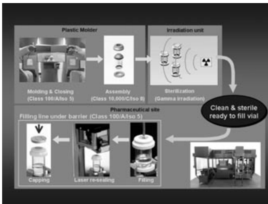
Figure 30.1 Overview of the closed vial technology process, including vial manufacturing, vial sterilization and vial filling
