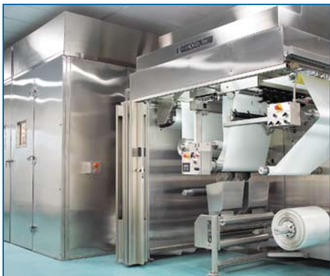
Final wind station equipped with on-line vision system
