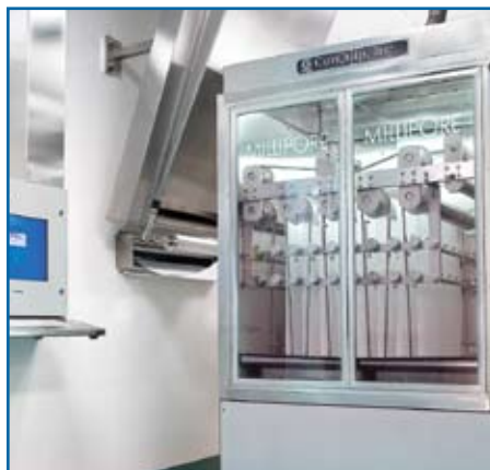
Temperature and flow control assure trace solvent removal from membrane prior to drying
