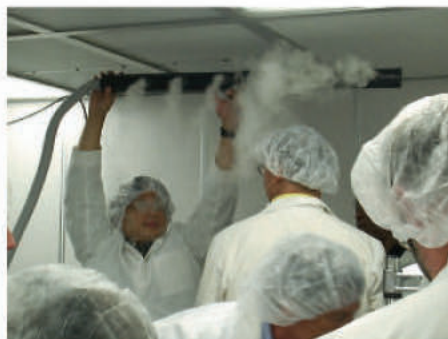
The difference in airflow from HEPA filter face and non-HEPA area is demonstrated.
