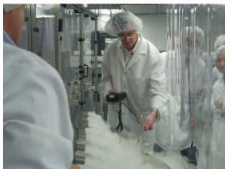
Airflow and velocity over the vial descrambler is tested.
