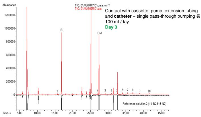
Contact with cassette pump and extension tubing – single pass-through pumping @ 100 mL/day
