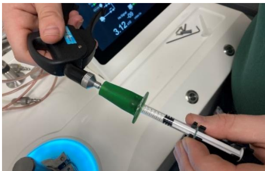
Tracer Gas Charging
