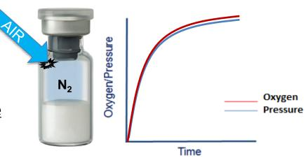
Understanding gas flow enables development of CCI test methods based on gas ingress
