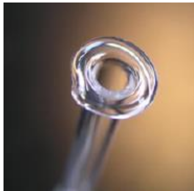
Fingertip not properly tooled
