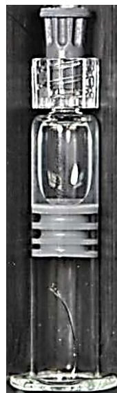
Crack not touching the drug
