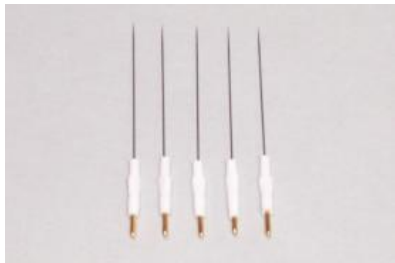
Tungsten needles for particle picking
