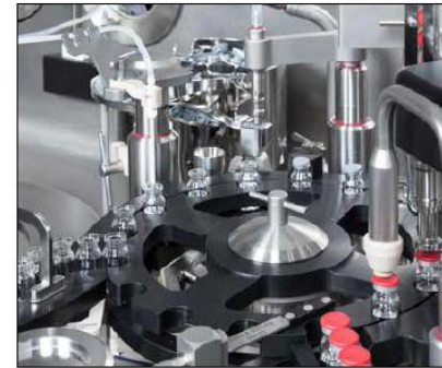
KSF 5105 – Fully automatic vial filling and closing
