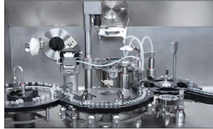
KSF 5105 – Fully automatic vial filling and closing
